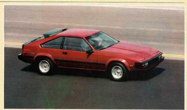
ics, though. The Celica Supra registered a drag coefficient of 0.35 in Japanese wind tunnels, a 14 percent improve-
